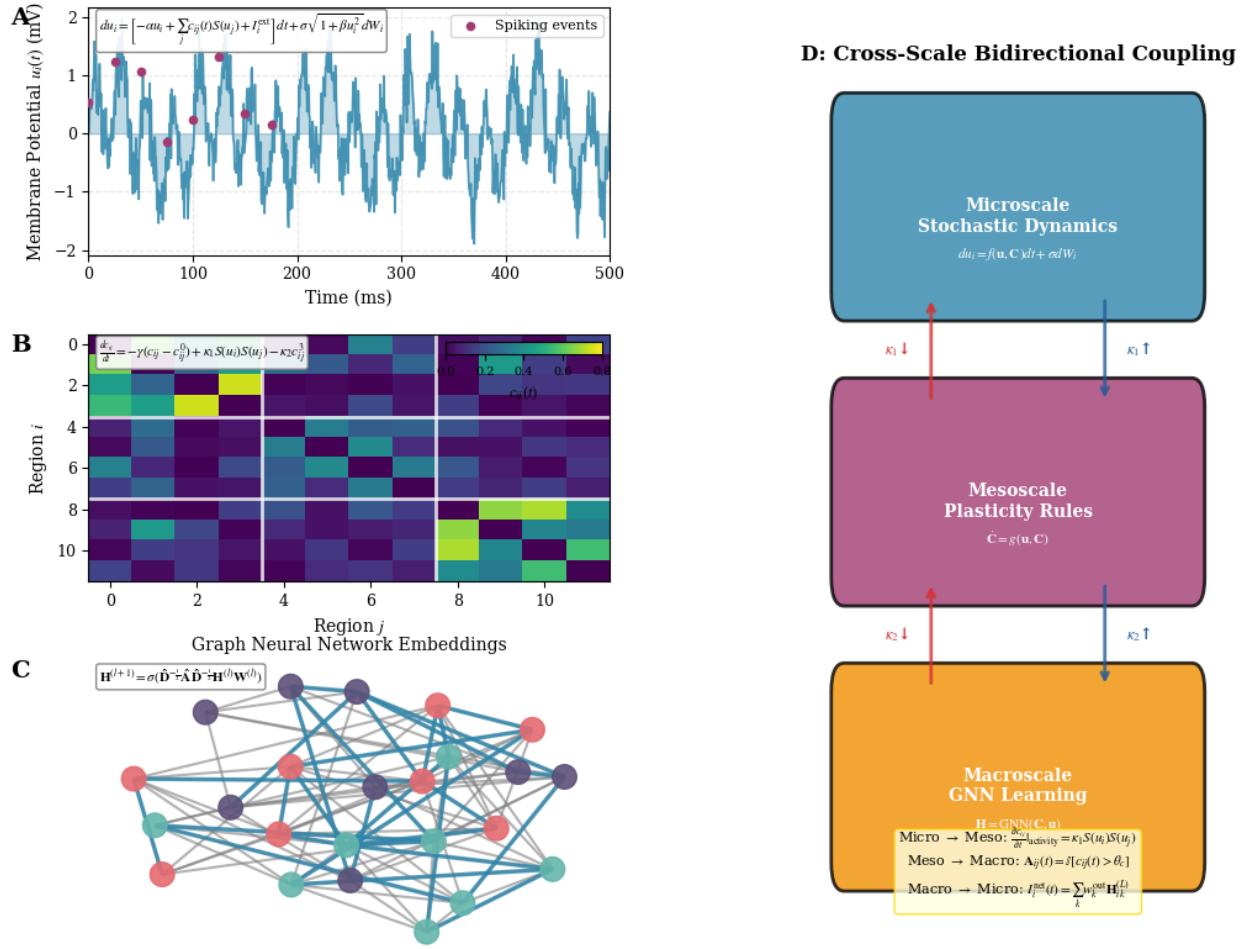
FIGURE 1. Multi-scale architecture of the proposed framework. (A) Microscale neural dynamics governed by stochastic differential equations with state-dependent noise. (B) Mesoscale dynamic connectivity matrix evolution through activity-dependent plasticity rules. (C) Macroscale graph neural network capturing emergent network properties. (D) Bidirectional cross-scale coupling enabling information flow between all hierarchical levels, creating closed feedback loops essential for emergent criticality and hierarchical temporal organization. The framework integrates stochastic dynamics at the microscopic level, synaptic plasticity at the mesoscopic level, and network learning at the macroscopic level.
